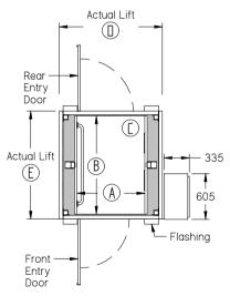
B MODEL - Dual Car Entry ELEVATION
